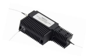
The OC Series 850nm MM Optical Circulators are non-reciprocal devices that redirect light at 850nm from port to port in only one direction while minimizing back reflection and back scattering in the reverse directions for any state of polarization. With Agiltron's special magnetic optics technology and proven micro optics design, the circulator features low insertion loss, high isolation, compact structure, high power handling, and high stability.
