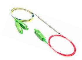
Agiltron's double-clad 2x2 fiber coupler combines a double-clad fiber (single mode core surrounded by a multimode inner cladding) with a large core multimode fiber. Light in the single mode core of the double-clad fiber (DCF) is guided through the coupler with little loss ( $\leq$ 0.5 dB). Light in the multimode inner cladding of the DCF is transferred to the output multimode fiber with  $\geq$ 60% transmission.
