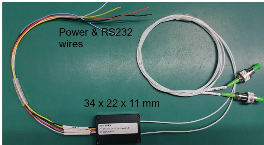
Figure 1 Ports of EDFA
