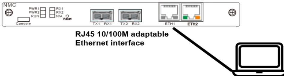
Use Twisted pair cable to connect ETH1 or ETH2 with your computer and configure the device and computer in the same IP segment, then type the IP address from the website banner in your computer to go into the WEB management interface, **WEB address: 192.168.1.200:8081, default user name for WEB: admin, password: admin.**
