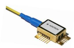
The AT10GC receiver consists of an avalanche photodiode, a low-noise preamplifier and a precision NTC thermistor in a hermetic coplanar package with a connectorized single-mode fiber pigtail. Differential outputs are provided to improve noise rejection for enhanced sensitivity. It has been optimized for use in 10Gb/s metro applications, either as a discrete device or within a transponder, using NRZ modulation, with or without FEC, at data rates up to 10.709 Gb/s.
