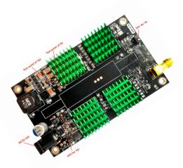
This NP series of fast-speed driver is designed to control the Premium NS series of solid state variable optic attenuators (VOA). The push-pull output design is especially suitable for driving capacitive VOA loads, assuring the fast response time both on rising and falling of attenuation. The VOA attenuation is controlled by 0-5V signal input. A wall plug power supply is provided for each driver.
