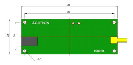
NOTE: When ordered with 100kHz driver, NSSW-2x2 will be mounted on this driver by soldering PINs on the PCB.
