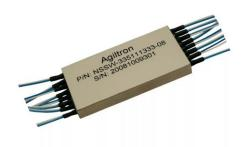
The High Speed Variable Fiber Optical Attenuator Array (NSAA) features fast response, ultracompact size, and low driving voltage. It controls laser power with channel number up to 48 in an integrated package. This is achieved using a special waveguide configuration. The response is about 100 to 300ns. Agiltron offers electronic driver with convenient 0-5V control input.
