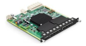
Support 2x40G or 2x100G signal service access. The main function is to convert the 2x40G or 2x100G with 3R regeneration to 2xWDM standard wavelength signal to multiplex different WDM wavelengths to transmit in the long haul. It is mainly used in 40G or 100G transmission networks.
