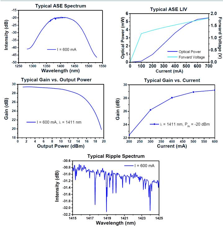
The sharp dips in the ripple spectrum are mostly caused by water absorption in the measurement setup.
