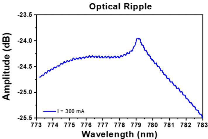
**Note:** The peak around 779 nm is from the OSA measurement setup (NOT from device)
