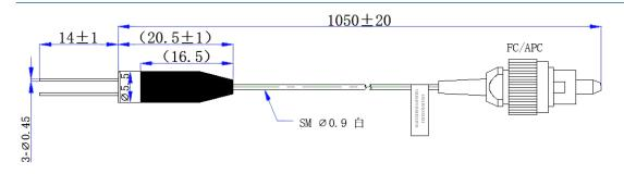
Standard Package for Infrared Band. For other wavelength band, size may vary due to special detector configurations.
